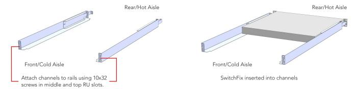
The SwitchFix does not ship in the fully extended position from the factory. Extend the SwitchFix by pulling evenly on the mounting rail tabs to the deepest depth.
